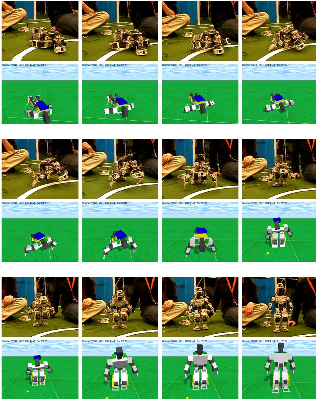
Figure 4.1: A first weak validation of the simulation: The stand up motion is keyframe-transition based and was developed on the real Bioid. The (raw) transfer of the identical keyframe structure to simulation shows similar behavior.
